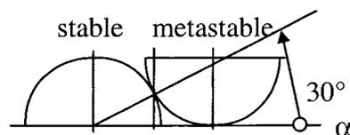
**Figure 6.** Vertical section of the arrangement of two hemispheres in alternate stable and metastable orientation.
