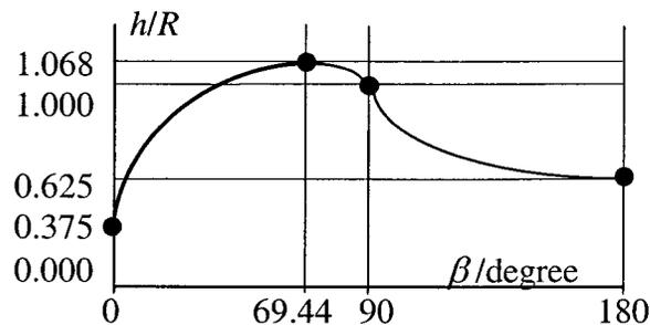
**Figure 2.** Diagram of the potential energy of a hemisphere in mg units as a function of the angle  $\beta$ .
