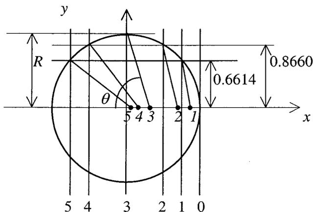
**Figure 3.** Projection of selected spherical sections on a plane through the axis. Roman numbers indicate the tangent (0) and cutting (1–5) planes; italic ones the centers of mass, shown by dots.
